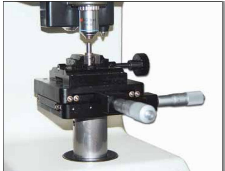
X-Y table 100 x 100 mm 0.01 mm division is included for easy location of test surface or Zig-Zag tests. OPTIONS: 2 Digital micrometers
