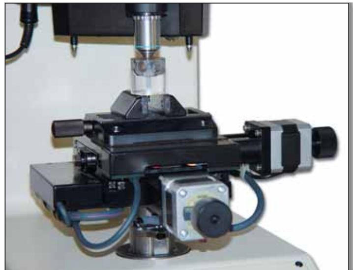
Motorised X-Y table connected with CNC computer for automatic tests
