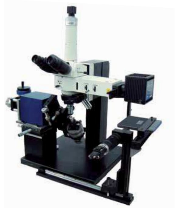
Measure of the geometry on Rockwell, Vickers indenters as per ISO 6508-3 ISO 6507-3
