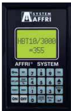
Optional: Automatic Brinell measure, for fast test on production department, it doesn't need any microscope
