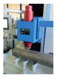
Automatic vertical stroke and programmable by PLC and automatic clamping test sample from any distance
