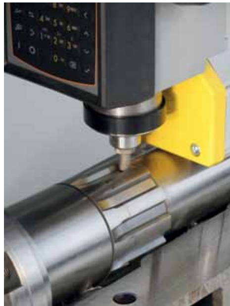
Vertical sliding indenter 50mm (2") range action assures easy test at different distance between test surface and indenter
