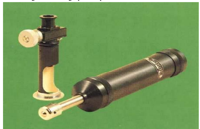
Fig. 1. Photograph of a portable Brinell hardness tester
